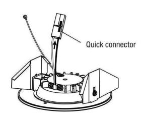
4. Connect the ground wire (yellow-green) by securing the terminal ring to the recessed housing using the provided self tapping screw. Use 1/8" drill bit to drill hole on the recessed housing. Plug in the male and female parts of the connector.
