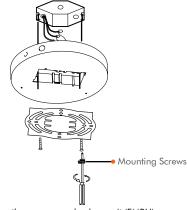
Screw the emergency backup unit (EMBU) into the junction box using the 2X8/32 screws provided. Then using the wire nut provided, connect the three (3) cables available for connection into junction box
