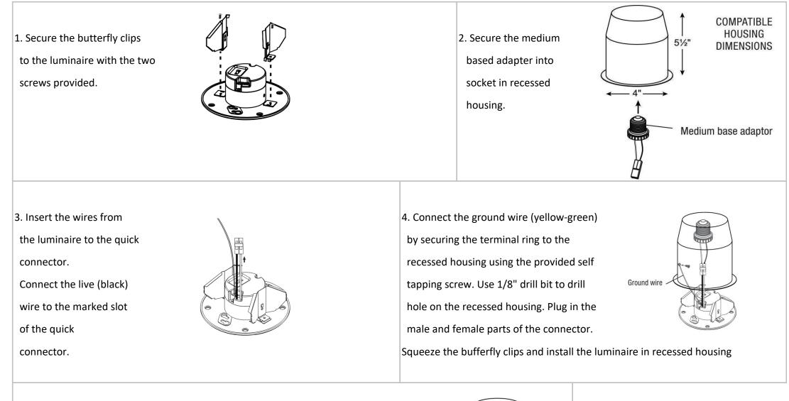
5. Center the luminaire in recessed housing.
